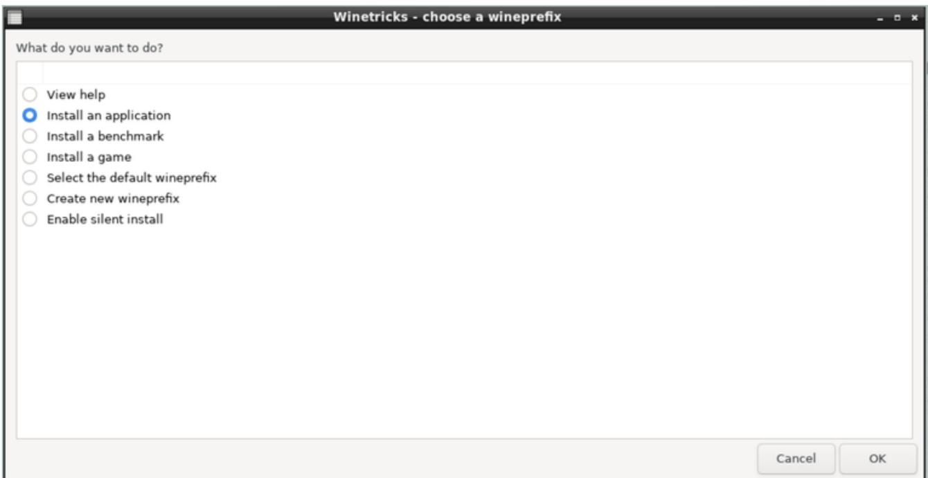
Selecting either *Install an application*, *Install a benchmark*, or *Install a game* shows a list with supported options, such as the one below for applications:
