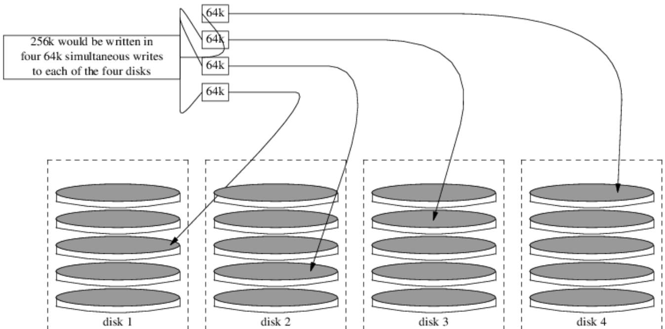
Each disk in a RAID0 stripe must be of the same size, since I/O requests are interleaved to read or write to multiple disks in parallel.
