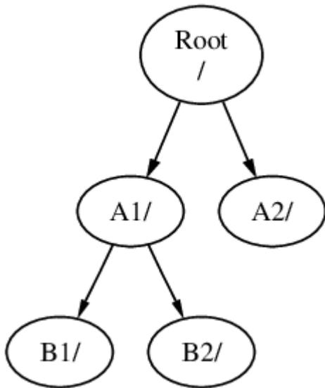
Any files that are in the **B1** or **B2** directories can be reached with the path **/A1/B1** or **/A1/B2** as necessary. Any files that were in **/A1** have been temporarily hidden. They will reappear if **B** is *unmounted* from **A**.
