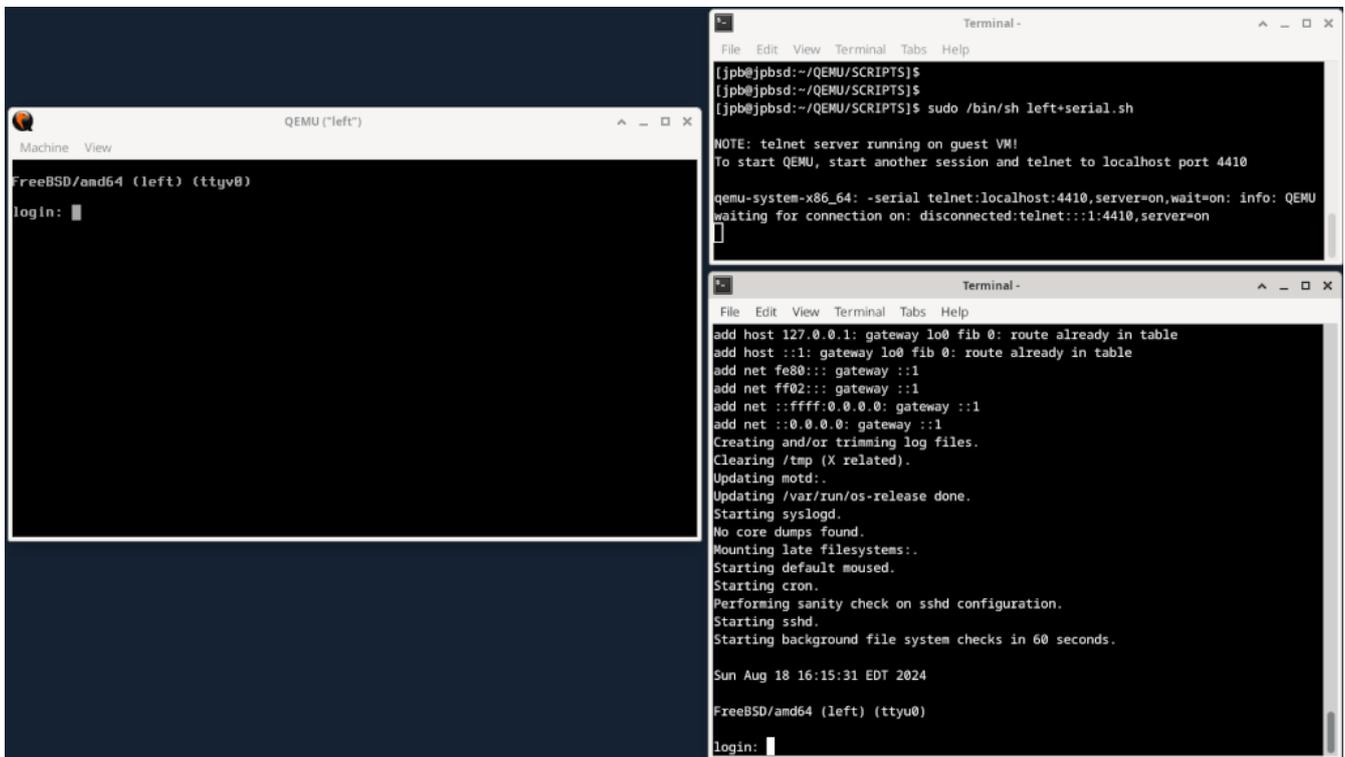
Figure 67. Enabling a Serial Port over TCP
