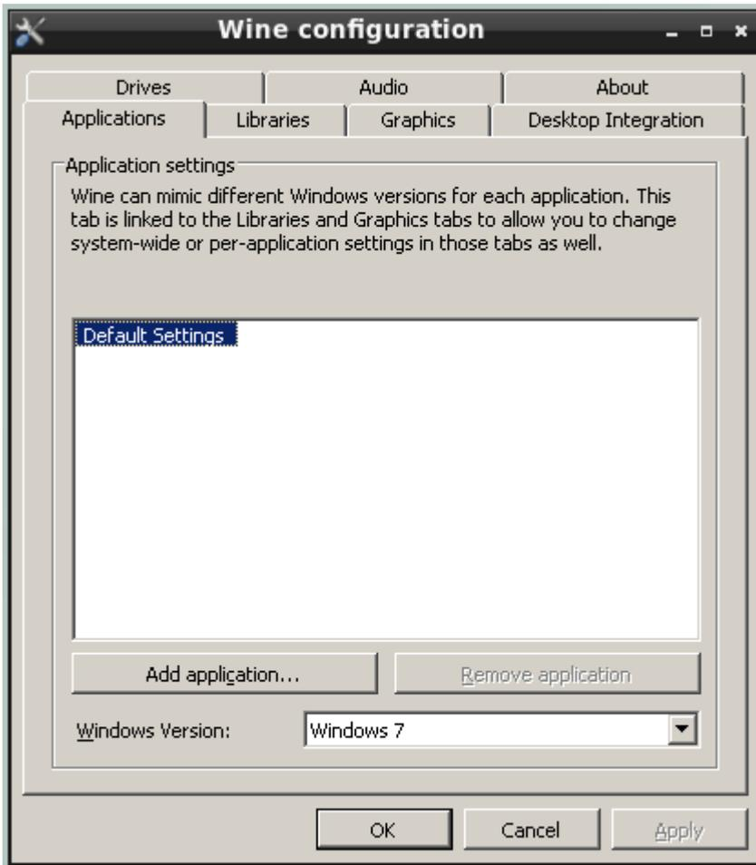
The *Applications* contains controls enabling the association of programs with a particular version of Windows®. On first start-up the *Application settings* section will contain a single entry: *Default Settings*. This corresponds to all the default configurations of the prefix, which (as the disabled *Remove application* button implies) cannot be deleted.
