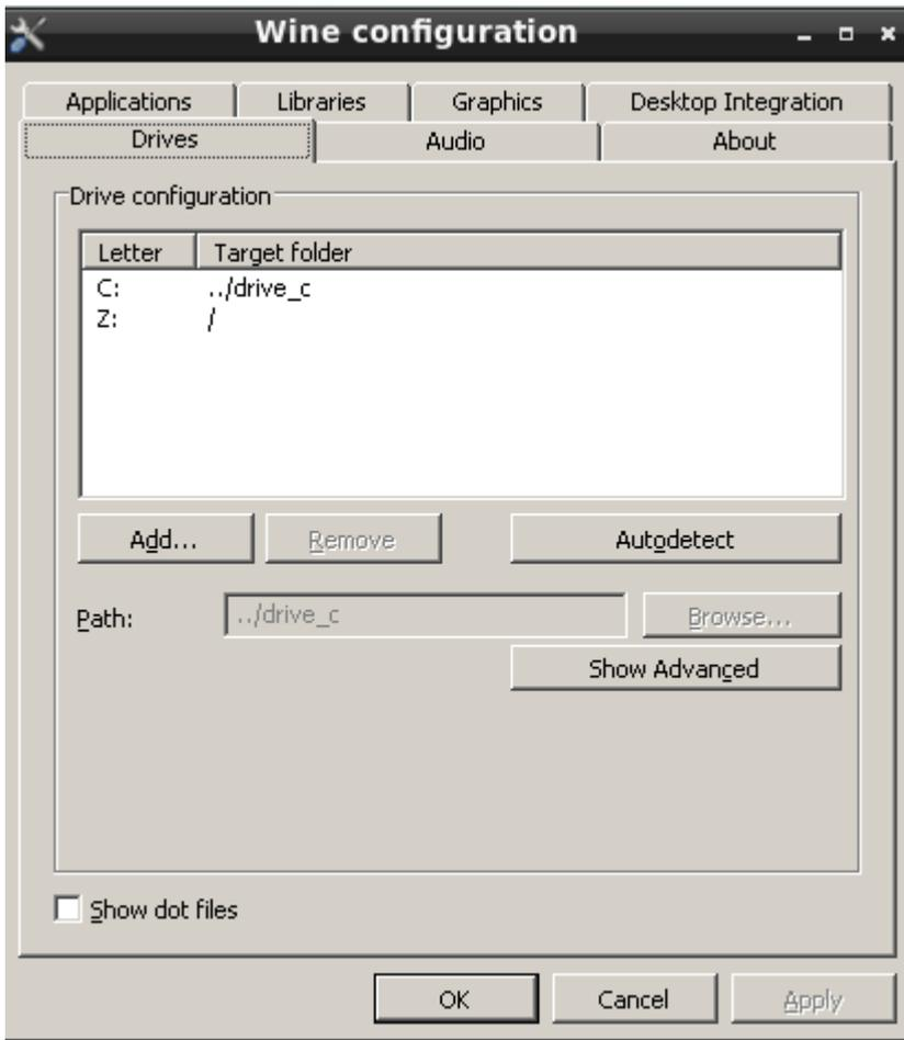
The *Drives* tab allows linking of directories in the host FreeBSD system to drive letters in the Windows® environment. The default values in this tab should look familiar, as they are displaying the contents of `dosdevices/` in the current WINE prefix. Changes made via this dialog will reflect in `dosdevices`, and properly-formatted links created in that directory will display in this tab.
