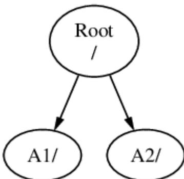
A file system must be mounted on to a directory in another file system. When mounting file system
